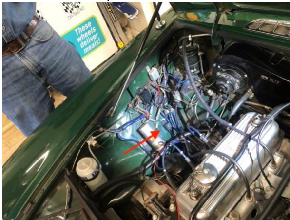
5 pin relay before it is mounted and grounded.
